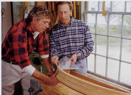
Templates are the key. For each section of beading, Lamb (right) made a plastic template directly from the elliptical table apron, and passed it on to Anderson (left).
