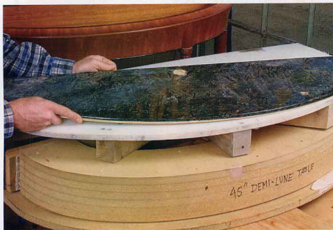
Another template for the inlaid tabletop. The plastic pattern was made from the apron's lamination form. Anderson used the template to rout the final profile of the top.
