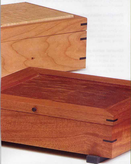
Sides resawn from thick stock on the bandsaw will produce a box with four matching corners.
