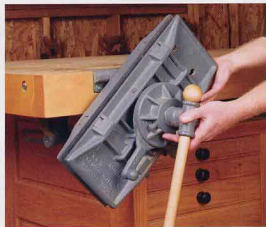
The jaws on an Emmert patternmaker's vise adjust in three planes, a feature that can prove useful when clamping odd-shaped parts. The jaws rotate 360° (left), pivot 90° (center) and taper (right).
