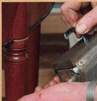
Round sections for round legs. Anderson made these bead sections, which mirror the projection of the leg turrets, by turning a flat stone disc, removing the center, cutting off a section and mitering the ends to fit the adjacent beads. A few strokes on an oilstone fine-tuned the fit of one mitered end to another. These circular beads were epoxied into place.
