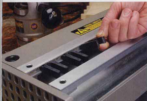
Locking fingers. The finger templates on the Akeda lock onto the jig's back rail, allowing for easy and precise adjustments.
