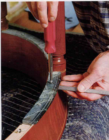
Attaching the bead sections. Each section was screwed to the apron; the rubber washers distributed the pressure gently. Care was taken to maintain an even projection from the apron.
