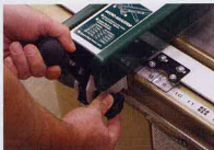
Dialing for precision. The HTC rip fence, a Biesemeyer look-alike, has a feature you won't find on the Biesemeyer: a dial that allows the fence to be micro-adjusted.
