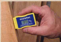
Small but effective. The Moistec moisture meter is small enough to fit into a pocket, making it easy to bring along when buying wood at the lumberyard.
