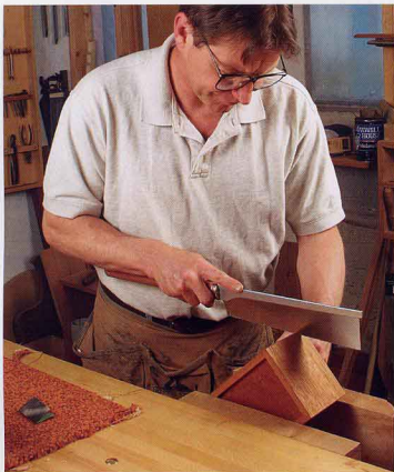
Hand-cut key slots. Use a backsaw to cut diagonally into the corner. Make sure the depth of cut is even on both sides.
