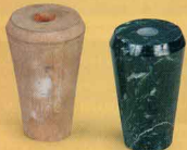
Precise pattern for the feet. Anderson used a turned wooden mock-up of a foot as a template. By mounting a right-angle grinder (armed with a diamond wheel) in the tool post of an old metal lathe, Anderson created a stone-turning machine.
