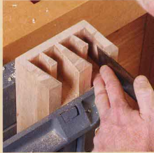
Cut the pins. Use a Forstner bit to remove most of the waste material from the pin ends. A chisel takes care of any waste that remains.
