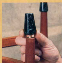
A strong leg-to-foot joint. Lamb used a dowel, epoxy and the same mandrel hole used for turning the stone feet to attach each one permanently.
