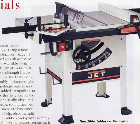
New 10-in. tablesaw. The Supersaw from Jet is shown here with the optional sliding table.
