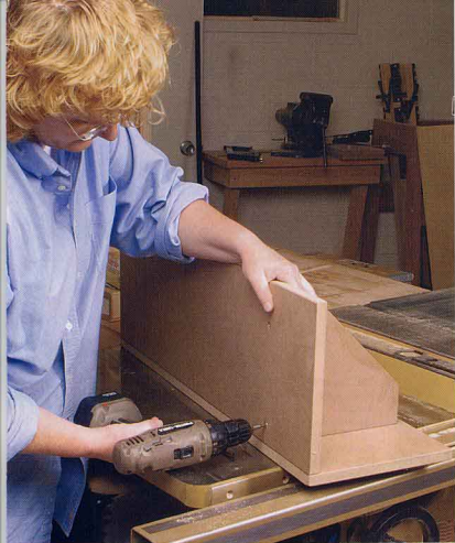
Modern screws like man-made materials, too. With sharp, coarse threads, modern screws work better than traditional screws in MDF, particleboard and plywood.
