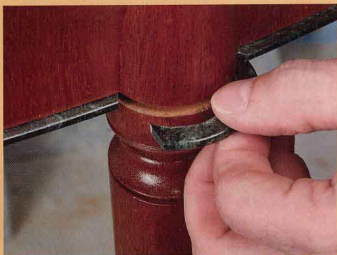
Round sections for round legs. Anderson made these bead sections, which mirror the projection of the leg turrets, by turning a flat stone disc, removing the center, cutting off a section and mitering the ends to fit the adjacent beads. A few strokes on an oilstone fine-tuned the fit of one mitered end to another. These circular beads were epoxied into place.
