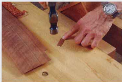
Tenderized veneer. If the veneer spline is too thick to slide into the sawkerf, a few hammer blows will persuade it to fit.
