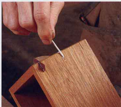
Thin but strong. Despite its flexibility, the long-grain to long-grain glue bond strengthens the whole joint.
