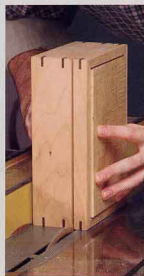
2. Partial cut. Lower the blade to leave \frac{1}{8} in. of wood on the short sides. This alleviates clamping or supporting the lid with shims during the final cut.
