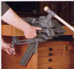
The jaws on an Emmert patternmaker's vise adjust in three planes, a feature that can prove useful when clamping odd-shaped parts. The jaws rotate 360° (left), pivot 90° (center) and taper (right).
