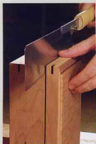
3. Final cut. Use a hand-saw to cut through the two short sides. Clean up the edges of the box and the lid with a block plane.
