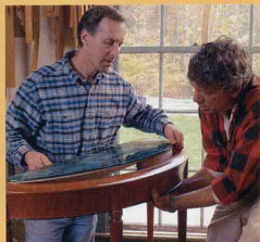
Attaching a stone tabletop. After laying on a coat of auto-body filler and running the tabletop slab through a wide-belt sander to create uniform thickness, Lamb and Anderson glued blocks to the bottom of the slab with epoxy. The blocks, in turn, were screwed to the apron.
