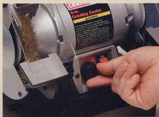
Low-cost grinders with speed control. The Craftsman 21152 (shown) and Delta GR250 bench grinders allow you to vary the speed from 2,000 rpm to 3,450 rpm simply by turning a knob.
