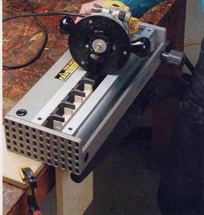
Dovetailing simplified. A new jig, called the Akeda, creates snug-fitting dovetail joints in relatively short order.
